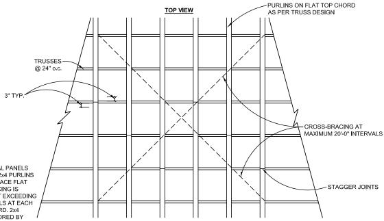
NOTE: IN LIEU OF STRUCTURAL PANELS (PLYWOOD SHEATHING) USE 2x4 PURLINS AS PER TRUSS DESIGN TO BRACE FLAT TOP CHORD. 2x4 CROSS BRACING IS REQUIRED AT INTERVALS NOT EXCEEDING 20'-0". USE 2 - 3" COMMON NAILS AT EACH CROSSING OF FLAT TOP CHORD. 2x4 PURLINS MAY ALSO BE ANCHORED BY EXTENDING THE PURLINS TO THE LAST HIP TRUSS IN A HIP SET CONNECTED TO THE ROOF DIAPHRAGM.
