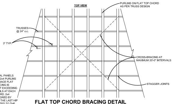
NOTE: IN LIEU OF STRUCTURAL PANELS (PLYWOOD SHEATHING) USE 2x4 PURLINS AS PER TRUSS DESIGN TO BRACE FLAT TOP CHORD. 2x4 CROSS BRACING IS REQUIRED AT INTERVALS NOT EXCEEDING 20'-0". USE 2 - 3" COMMON NAILS AT EACH CROSSING OF FLAT TOP CHORD. 2x4 PURLINS MAY ALSO BE ANCHORED BY EXTENDING THE PURLINS TO THE LAST HIP TRUSS IN A HIP SET CONNECTED TO THE ROOF DIAPHRAGM.
