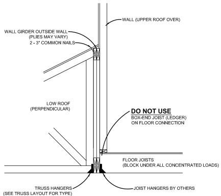
WALL GIRDER OUTSIDE, ROOF PERPENDICULAR, FLOOR PERPENDICULAR
