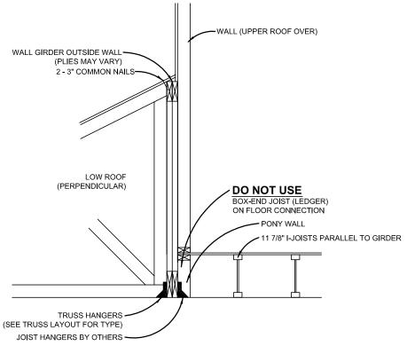
S WALL GIRDER OUTSIDE, ROOF PERPENDICULAR, FLOOR PARALLEL NOT TO SCALE
