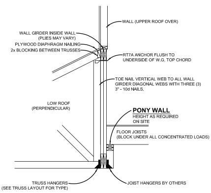
WALL GIRDER INSIDE, ROOF PERPENDICULAR WITH PONY WALL
