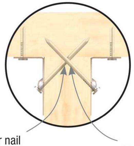
Double shear nail design features fewer nails and faster installation
